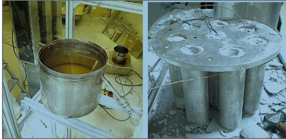
Figure:-2.8.5. Storage container and aluminum top with salts cylinders (22).
