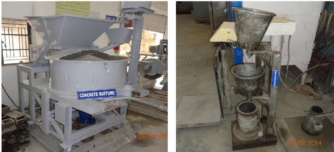
Figure: 3.2: Concrete mixer and compacting factor apparatus
