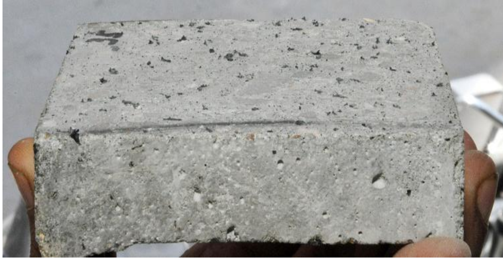
Figure 4.15: Surface of the rubberized concrete after abrasion test
