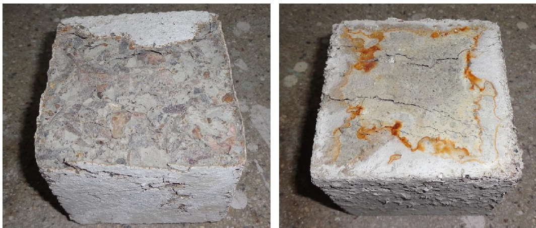
Figure 4.5: Failure pattern of control specimen and rubberized specimen after compressive loading
