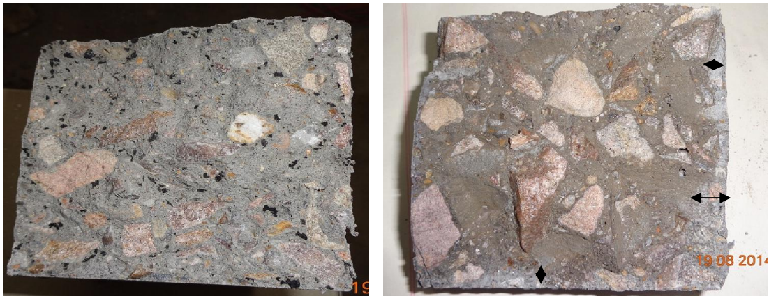
Figure 4.33: Freshly splitted concrete specimen and the control specimen showing depth of chloride penetration after 28 days (arrow shows depth of chloride penetration)
