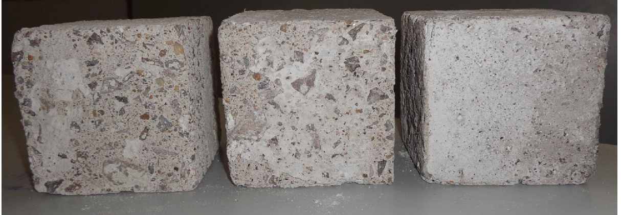
Figure 4.39: Images of acid attacked specimen at 28 days. The specimen with 0%, 10% and 20% crumb rubber
