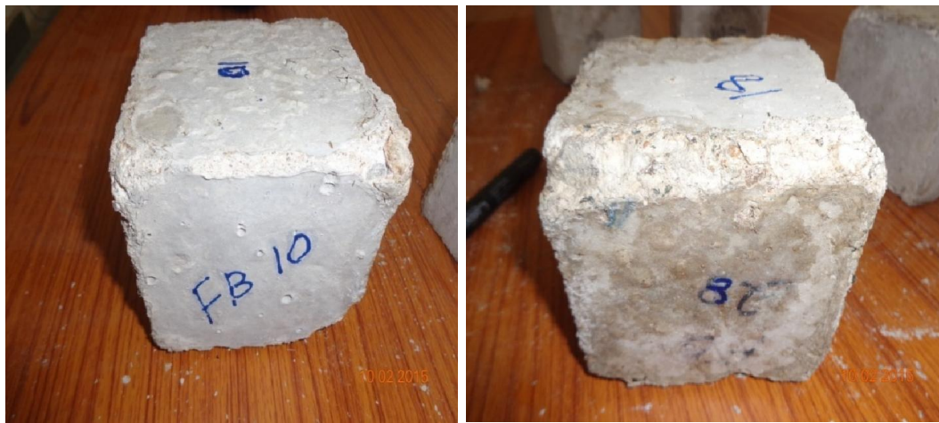
Figure 4.53: Control concrete specimens and rubberized specimen after 182 days of sulphate attack test
