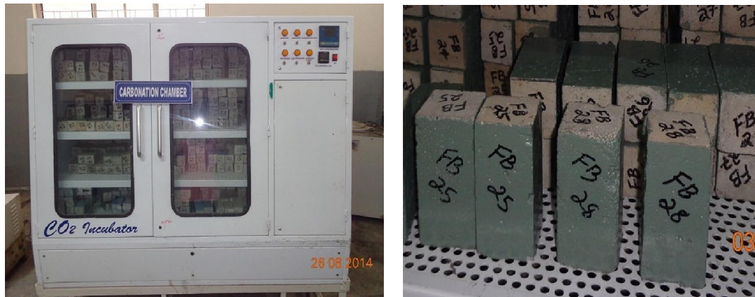
Figure 3.11: Carbonation chamber and epoxy coated concrete samples
