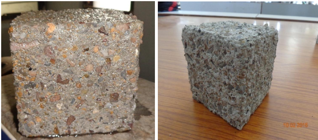
Figure 4.39: Images of acid attacked specimen at 28 days. The specimen with 0%, 10% and 20% crumb rubber
