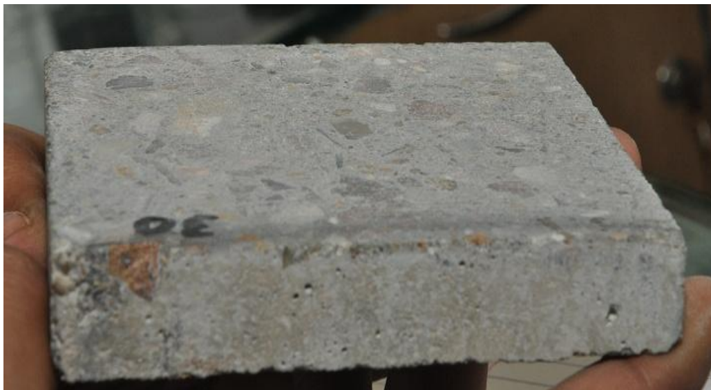
Figure 4.14: Surface of the control mix (with 0% crumb rubber) after abrasion test
