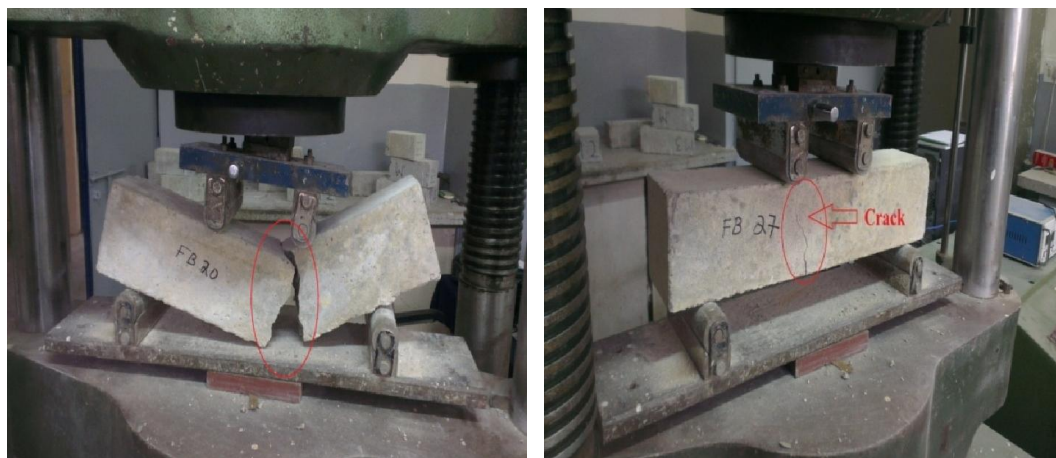
Figure 4.10 : Failure of control mix specimen and the specimen with 20% crumb rubber under flexural loading
