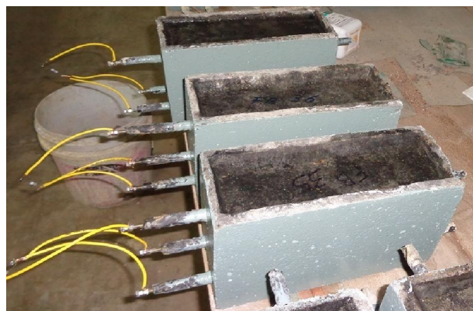
Figure 3.14: Epoxy coated specimens with 3% NaCl Solution
