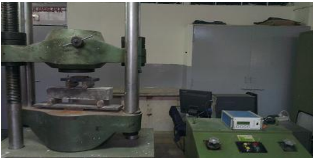
Figure 3.4: Flexural tensile strength testing on a universal testing machine
