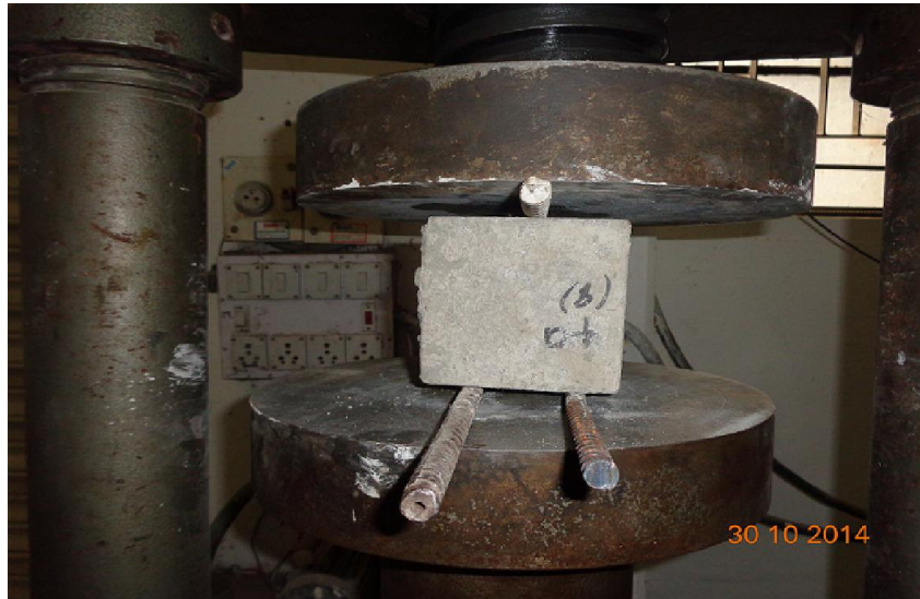
Figure 3.9: Splitting of concrete specimens to two halves
