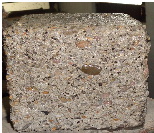
Figure 4.40 : Images of acid attacked specimen at 84 days. The specimen with 0%, 10% and 20% crumb rubber
