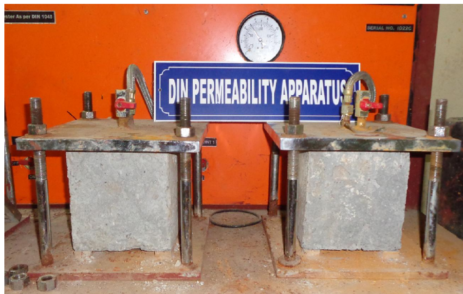
Figure 3.8: Water penetration apparatus as per din 1048
