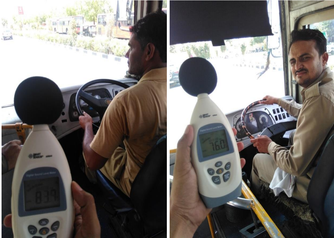
Figure 4: noise level measurement when driver was driving the bus
