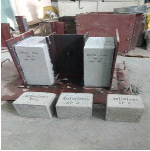
Fig. 3.16 After demolding of push-out test Specimen
