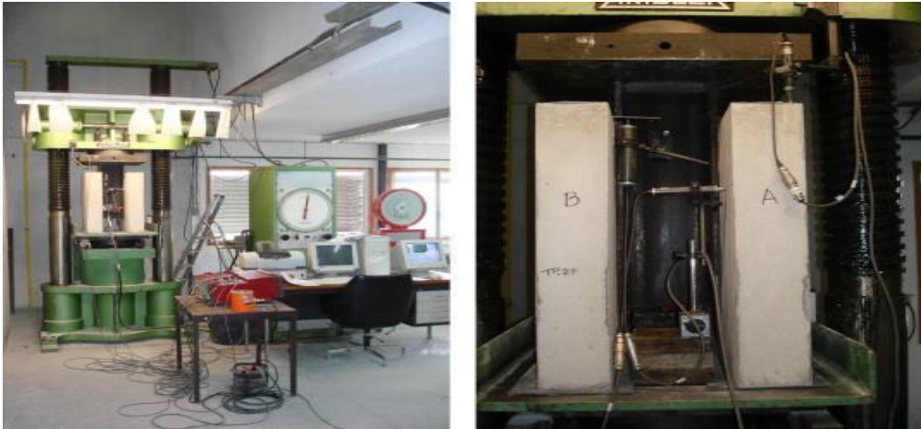
Fig. 1.6 Vertical Push out test arrangement ( Vianna et al. 2009 )
