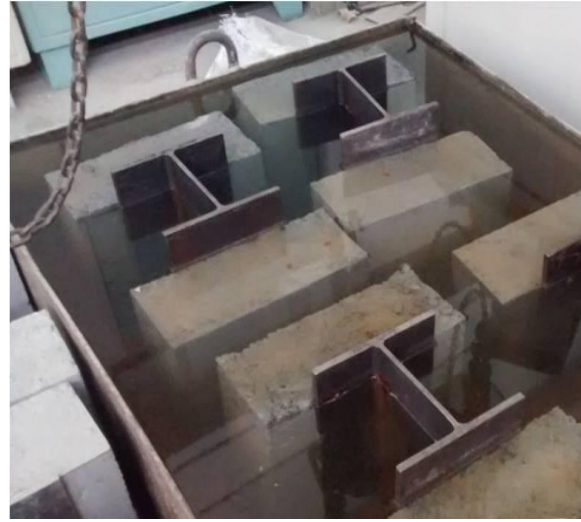
Fig. 3.17 Curing of Specimen
