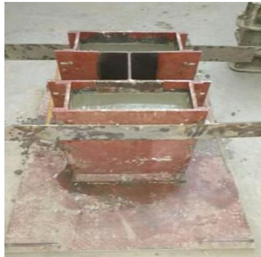
Fig. 3.15 Finished push-out test specimen
