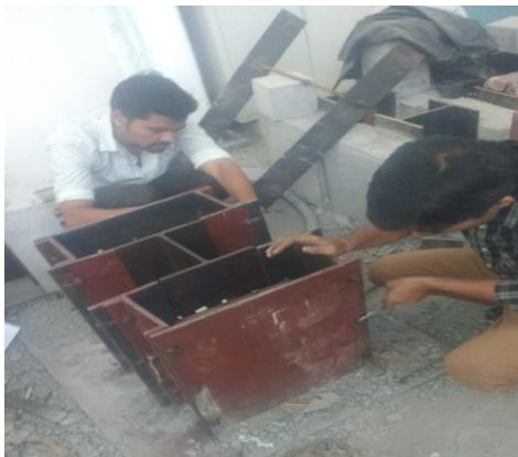
Fig. 3.2 Tightening of mould
