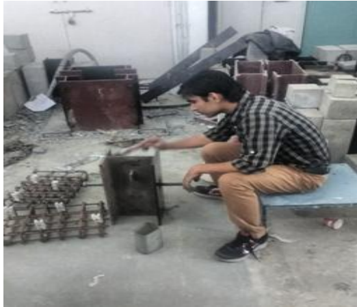
Fig. 3.12 Oiling of Steel section
