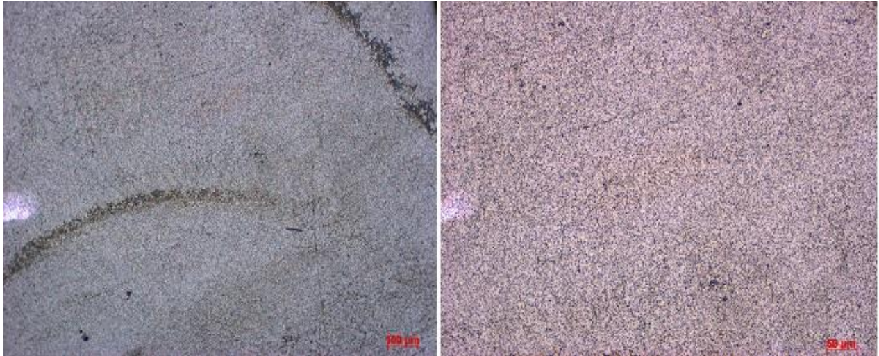
Figure 6: optical micrograph of Ti6Al4V surface etched with kroll's reagent.
