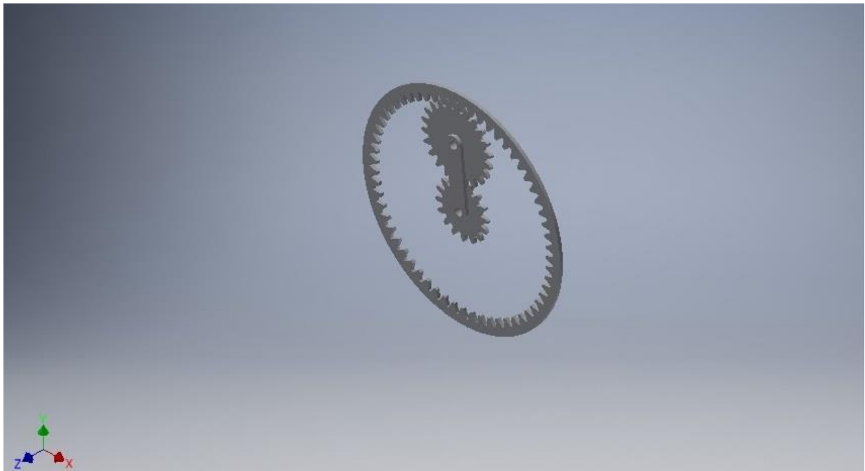
Figure 3.3: CAD model: Epicyclic Gear Set
