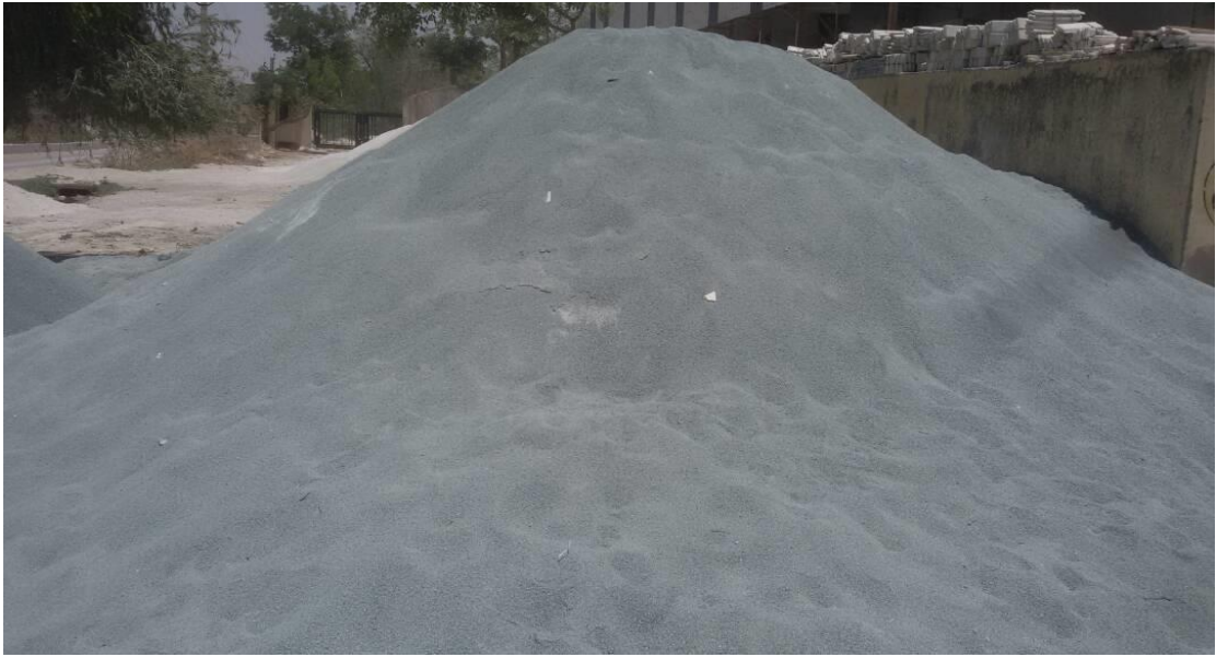
Image 3: Waste marble pieces are crushed to use with virgin concrete
