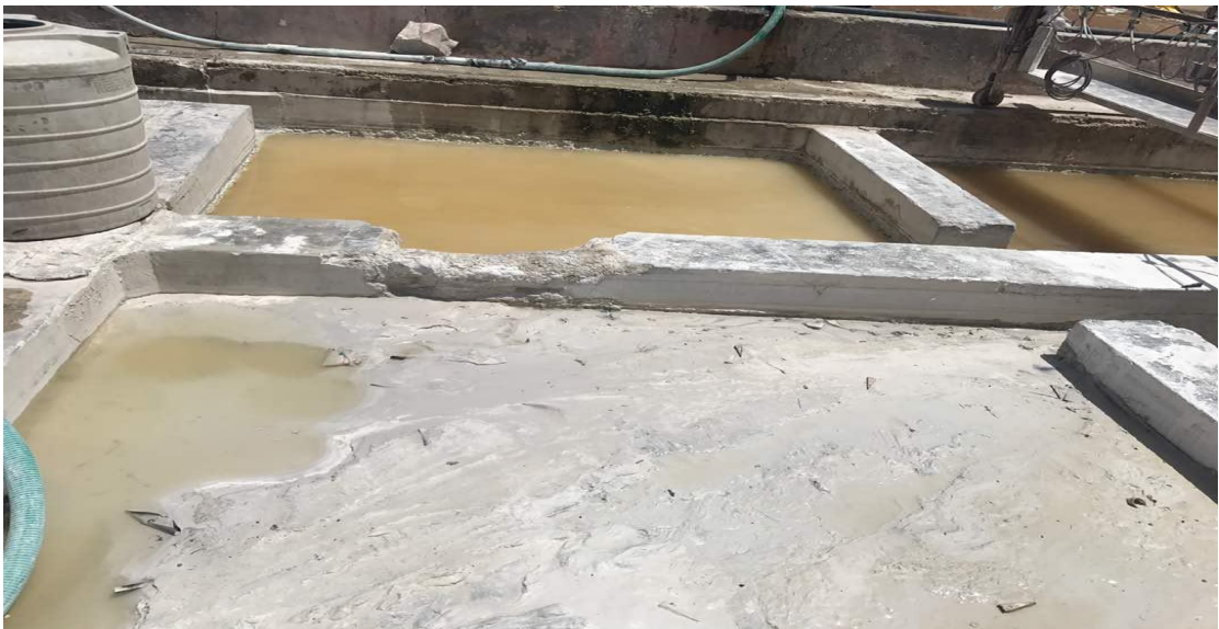
Image 2: Waste marble dust is being collected in tanks at plant site.
