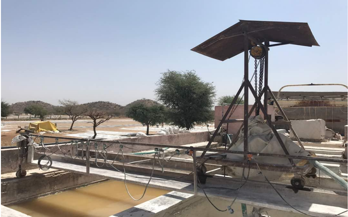
Image 1: Marble slurry/sludge collection plant (waste water also collected here)
