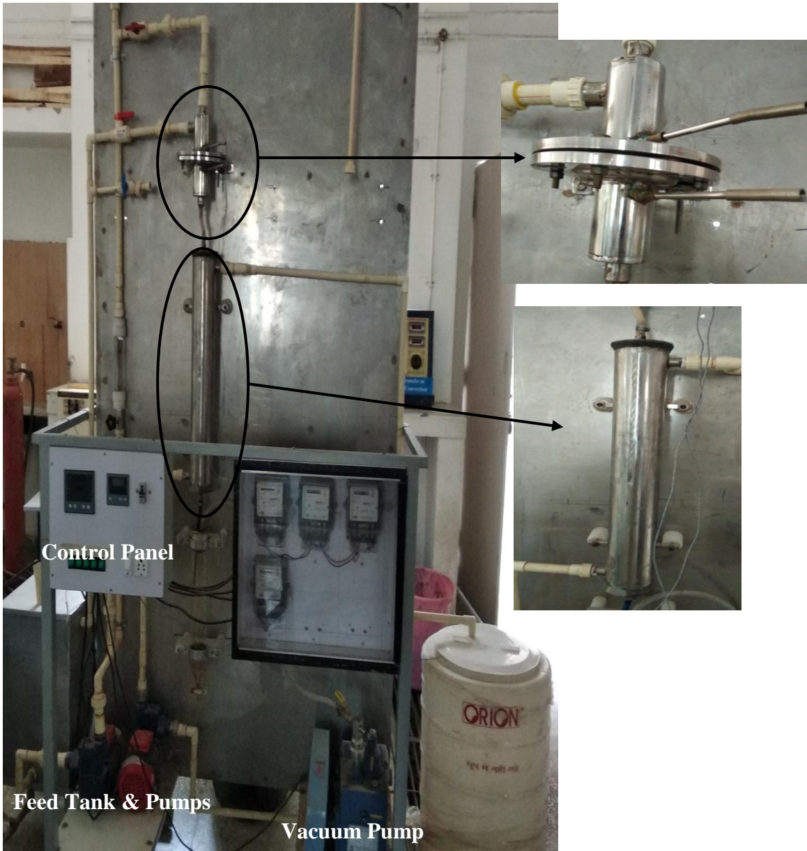
Figure 4.2: Pictorial diagram of lab scale vacuum membrane distillation unit
