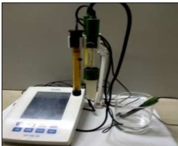
Fig. 3.15 Laboratory TDS analyser (HANNA, HI 5522)
