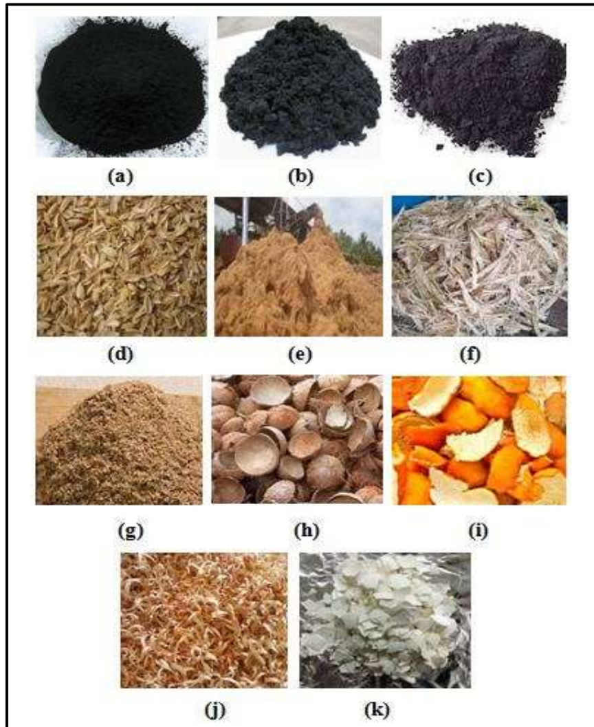
Fig 2.1 Commercial adsorbents (a) activated carbon (b) graphene (c) carbon nanotube and Bio adsorbents (d) rice husk (e) coconut coir pith (f) sugarcane bagasse (g) wheat bran (h) coconut shell (i) orange peel (j) saw dust (k) egg shell for chromium removal from wastewater
