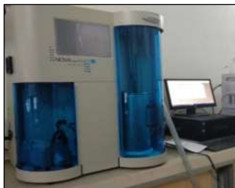
Fig. 3.8: BET surface area analyser (NOVA touch LX1)
