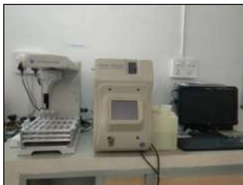
Fig. 3.14: Laboratory TOC analyser (Sievers InnovOx)
