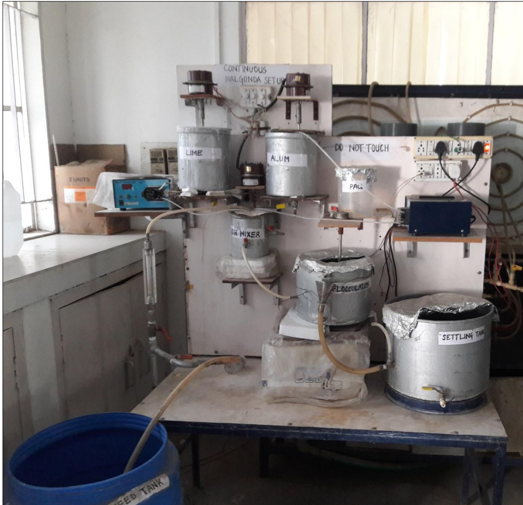
Figure 3.16 Pictorial view of continuous defluoridation set-up
