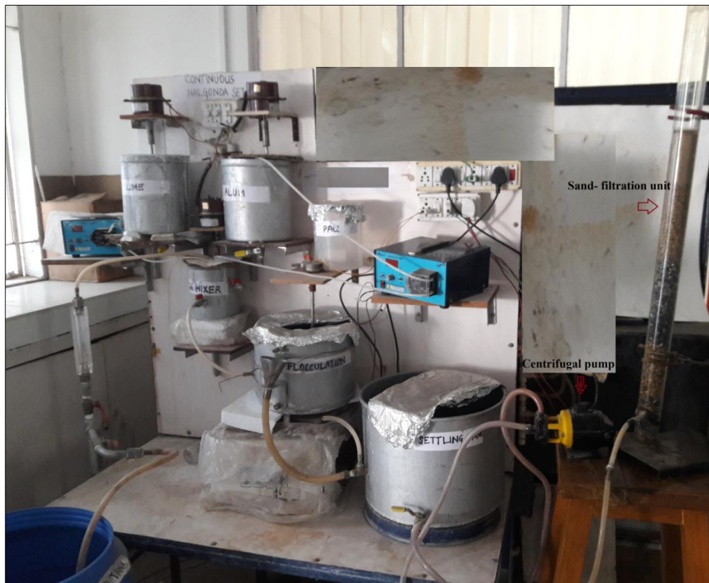
Figure 3.18 Schematic view of the sand filtration set-up
