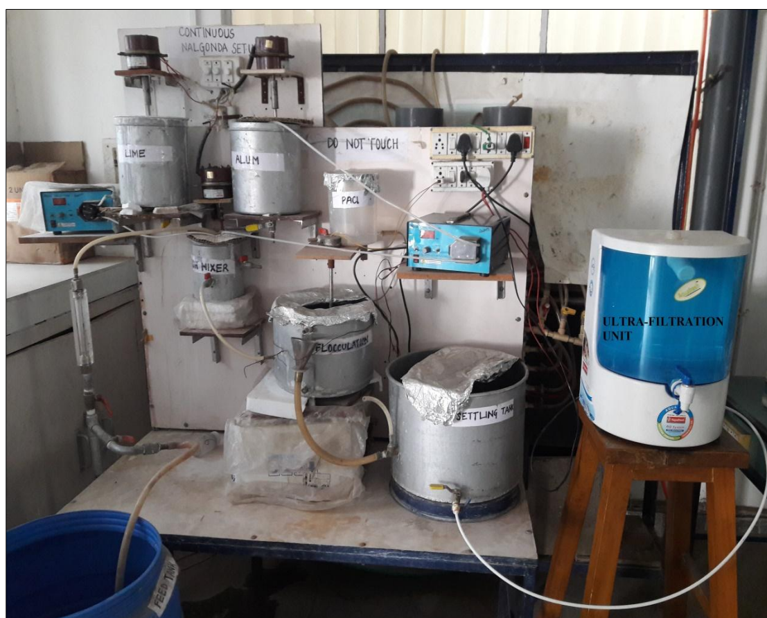
Figure 3.17 Pictorial view of continuous defluoridation set-up with ultra-filtration unit
