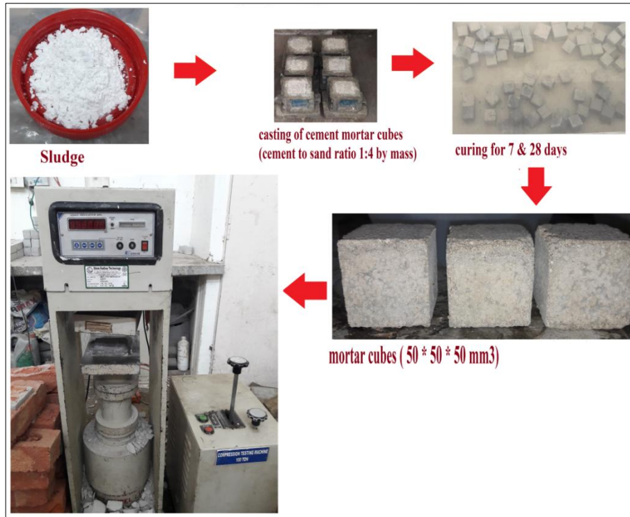
Figure 3.20 Process for Solidification of sludge
