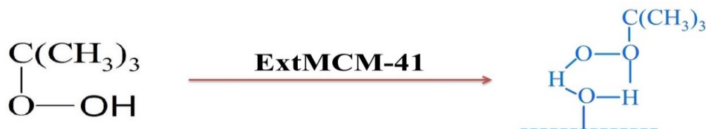
Scheme 4.3 Formation of 5 membered ring via coordination of TBHP and silanol group present on ExtMCM-41
