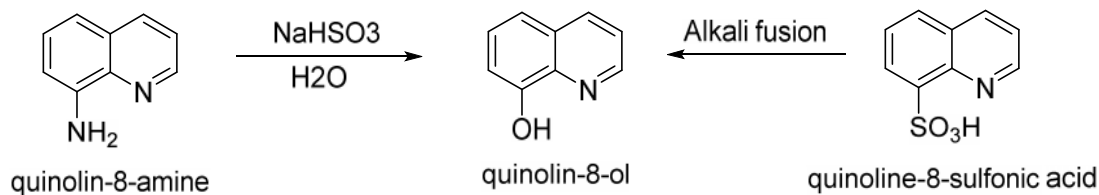
Scheme 1.2: Preparation of 8-hydroxyquinoline by diazotization and alkali fusion methods
