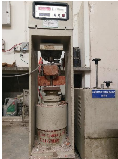
Fig. 3.14: Experimental setup to test tensile bond strength of mortars
