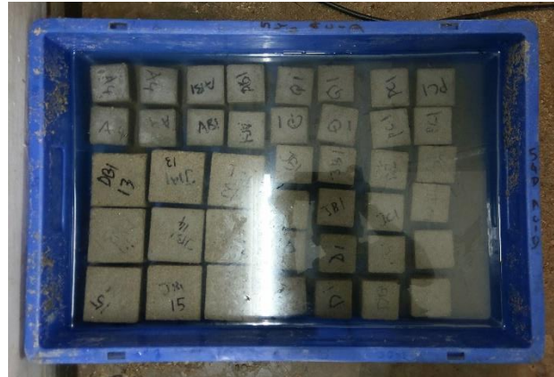
Fig. 3.18: Samples subjected to a 5% solution of sodium sulphate
