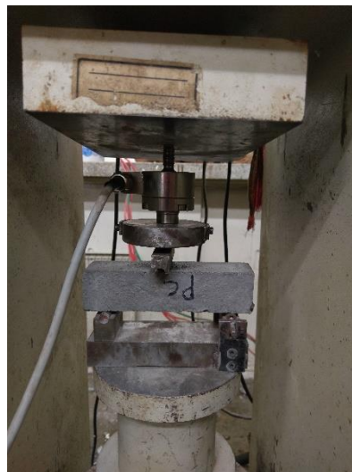
Fig. 3.13: Experimental setup to test flexural strength of mortars
