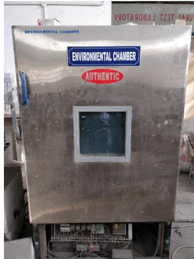
Fig. 3.20: Environmental chamber to simulate rapid freezing and thawing
