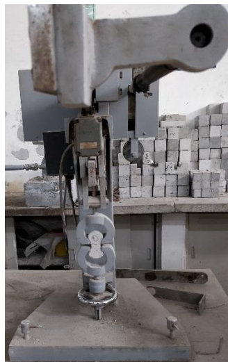
Fig. 3.12: Experimental setup to test tensile strength of mortars
