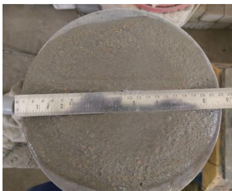
Fig. 3.9: Measurement of flow value of mortar mixes
