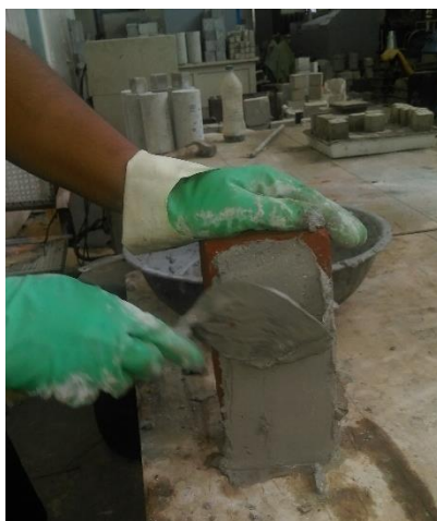
Fig. 3.15: Preparation of sample to test adhesive strength
