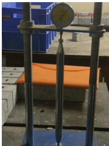
Fig. 3.16: Experimental setup to measure the length of mortar prisms
