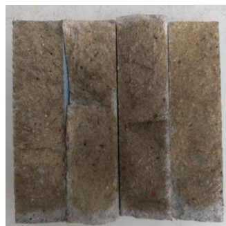
Fig. 3.21 Colour change when 0.1M solution of AgNO 3 is sprayed on samples soaked in NaCl
