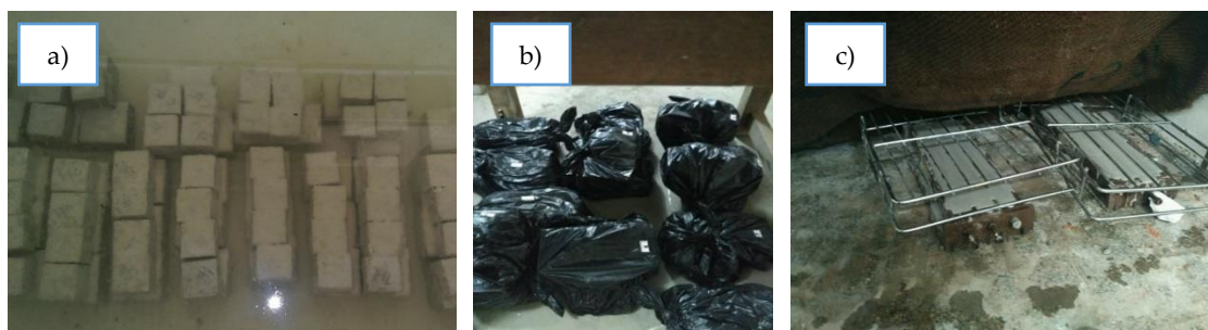
Fig. 3.8: Curing regimes: a) water curing; b) curing at ambient RH and temperature and c) moist curing
