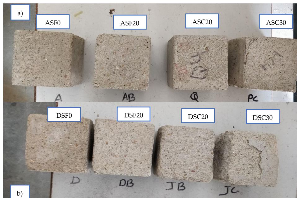
Fig. 4.47: Change in appearance of mortar mixes of series a) A and b) D after rapid freezing and thawing
