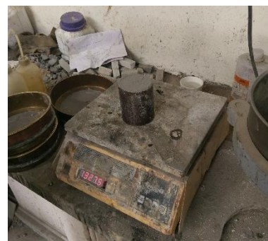
Fig. 3.10: Measurement of weight of fresh mortar mix in a standard container
