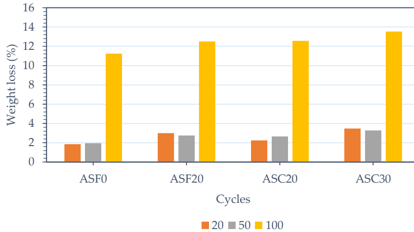
Fig. 4.46: Extent of weight loss suffered by mortar mixes of series A after rapid freezing and thawing
