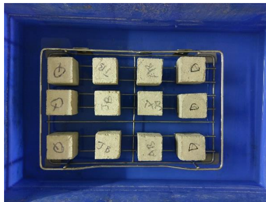
Fig. 3.17: Experimental setup to for conducting the capillarity test of mortar specimens
