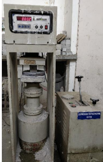
Fig. 3.11: Compression testing machine
