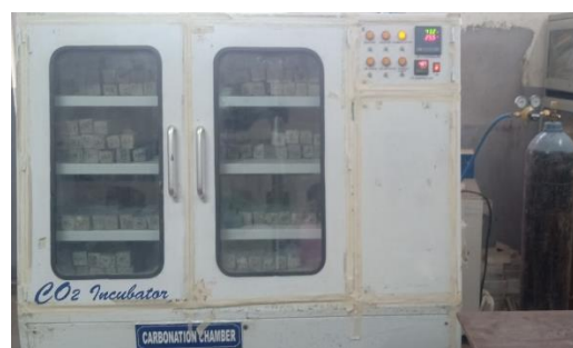
Figure 3.18 Specimen subjected to CO 2 in carbonation chamber
