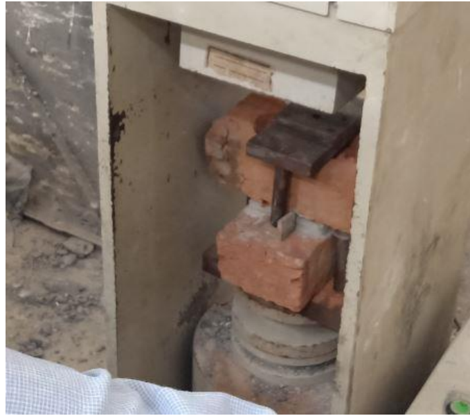
Figure 3.13 Testing of bricks couplet for bond strength test
