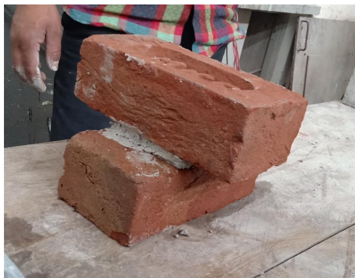
Figure 3.12 Casting of bricks couplet for bond test
