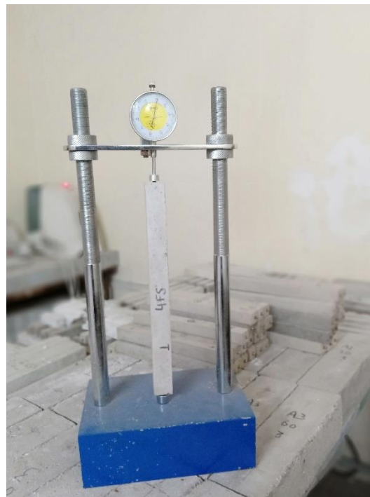
Figure 3.15 Drying shrinkage of cement mortar
