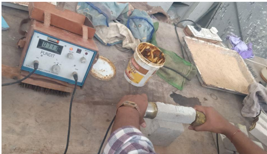
Figure 3.11 Experiment setup for UPV of mortar
