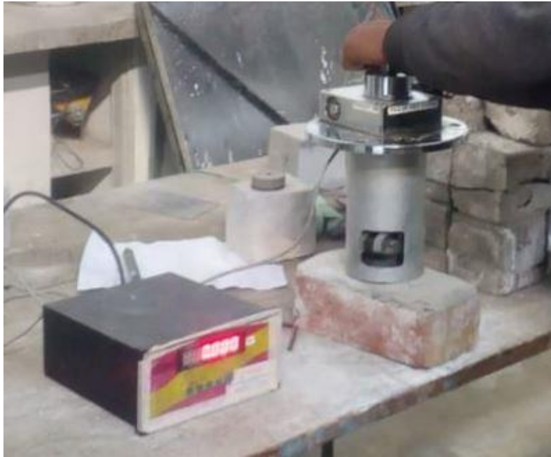
Figure 3.14 Testing of adhesive strength of cement mortar
