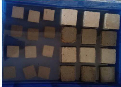
Figure 3.22 Specimens subjected to solution of sodium sulphate
