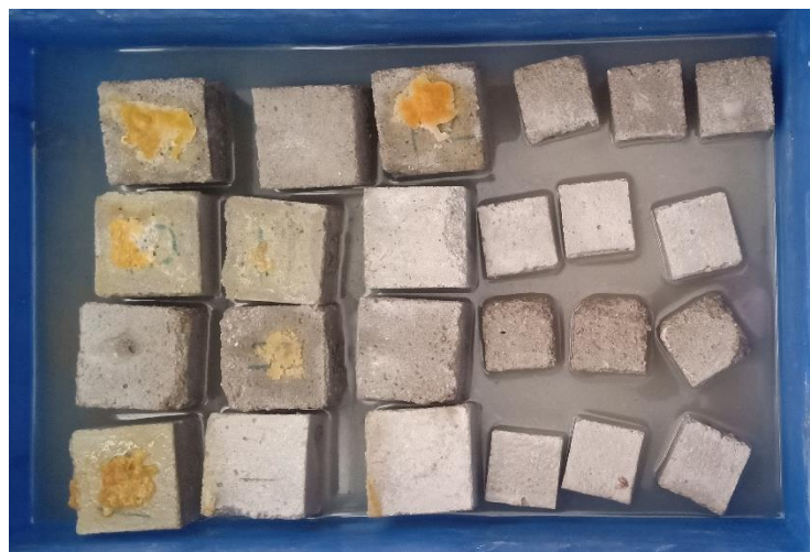
Figure 3.21 Specimens exposed to solution of sulphuric acid
