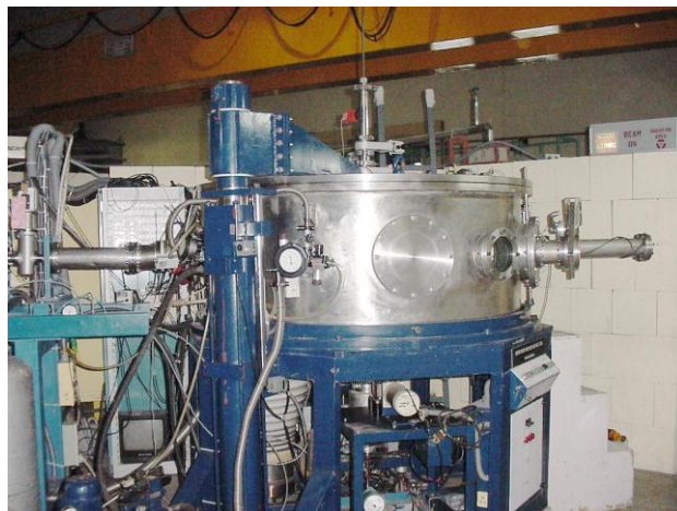
Figure 3.5 High vacuum irradiation chamber of Material Science beam line at IUAC New Delhi.
