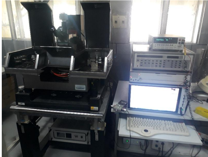
Fig. 6.17 Low level CV measurement of device at CSIR-CEERI.
