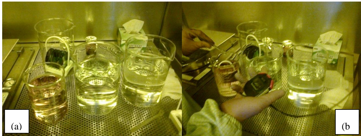
Fig. 5.12 (a) Developer CD26 (left) and two DI water beakers. (b) Developing UV exposed PR coated wafer in CD26 developer.
