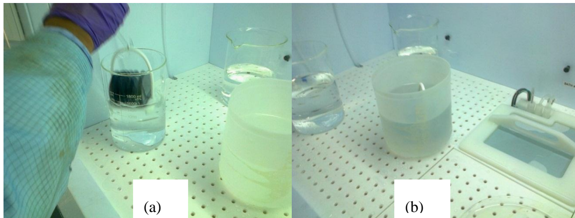
Fig. 5.8 (a) Piranha cleaning of wafers. (b) HF dip of wafers for oxide removal.
