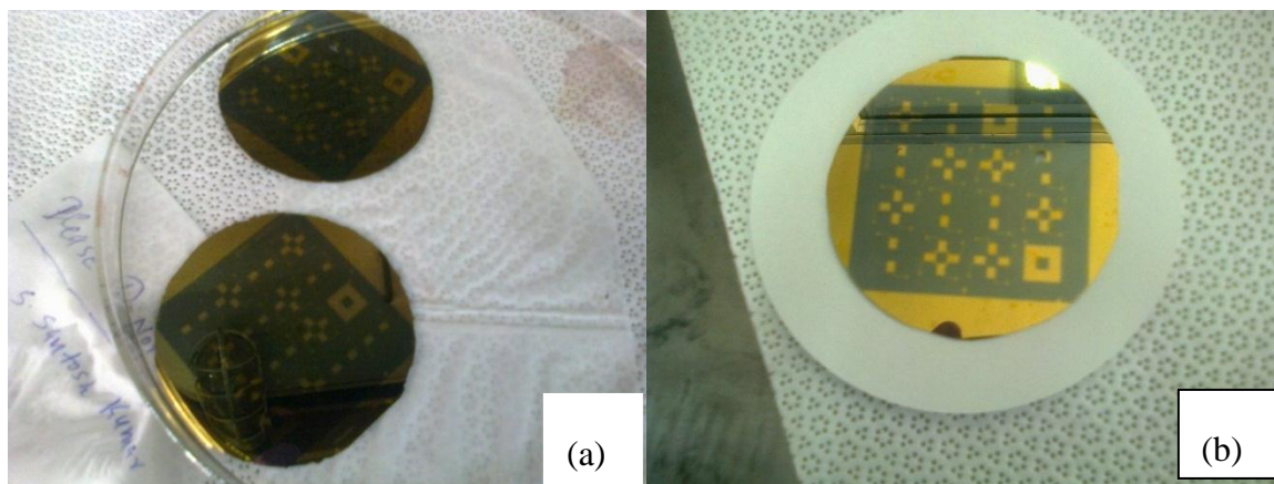
Fig. 5.17 (a) Chrome/gold etching of wafers. (b) Patterned bottom electrode wafer.
