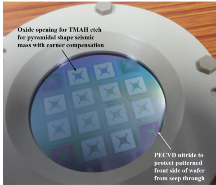
Fig. 5.26 Snapshot of the front side protection of the processed wafer with Zig for TMAH etching.
