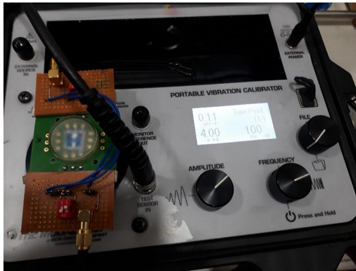
Fig. 6.25 Device mounted on 9100D Portable Shaker.
