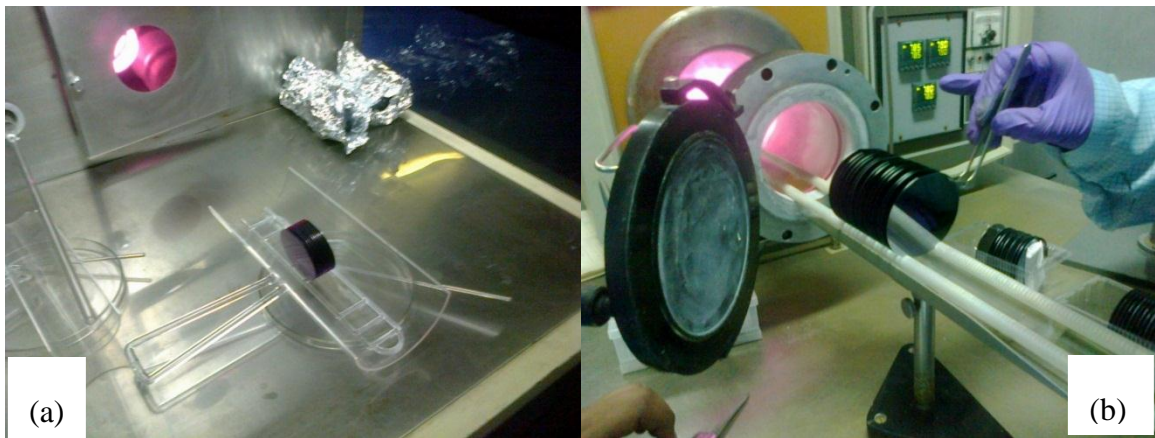
Fig. 5.9 (a) Wafers loading in thermal oxidation furnace. (b) Wafers loading in LPCVD nitride furnace.
