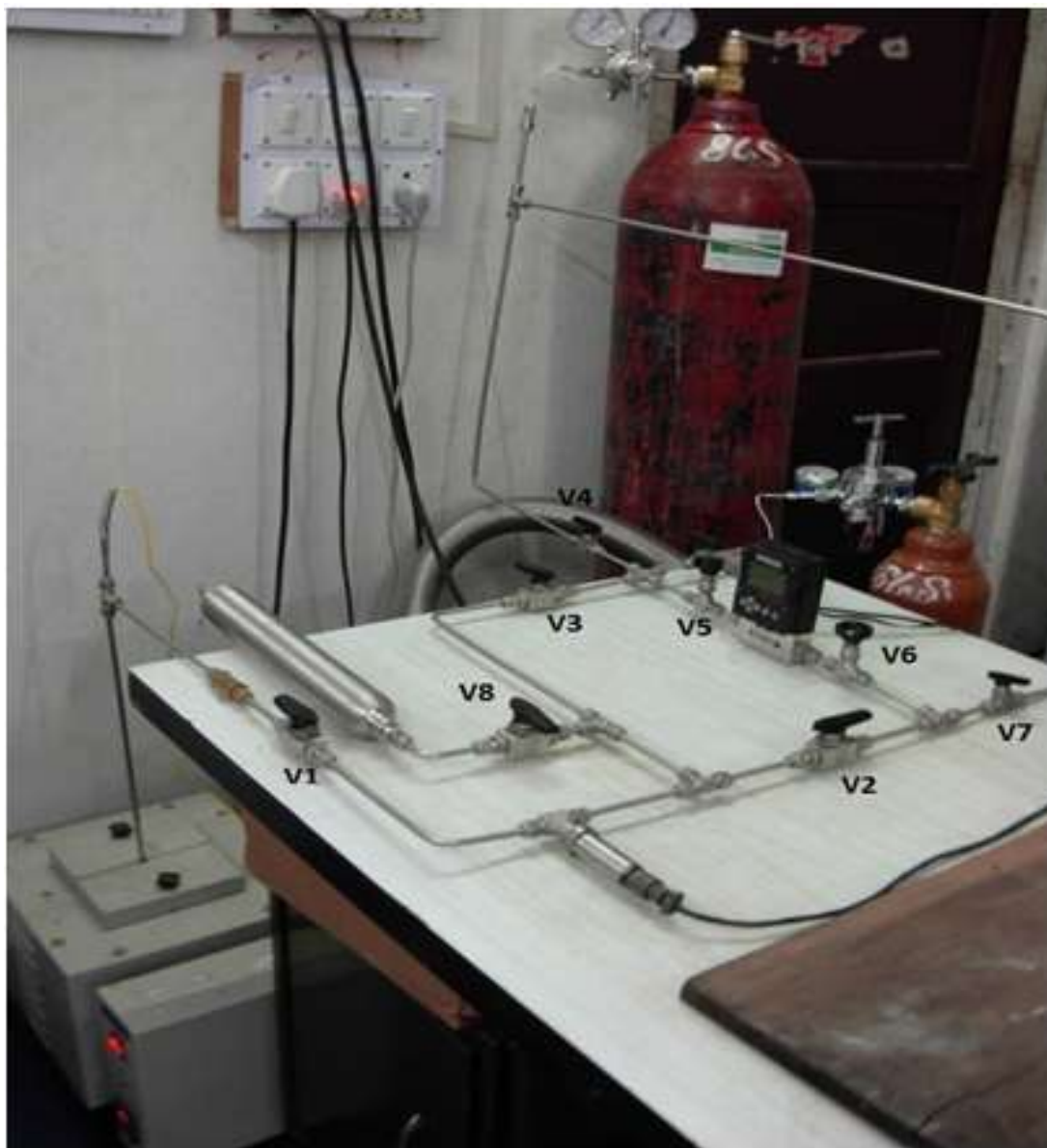
Figure 3.15. Experimental set up of hydrogen absorption and desorption
