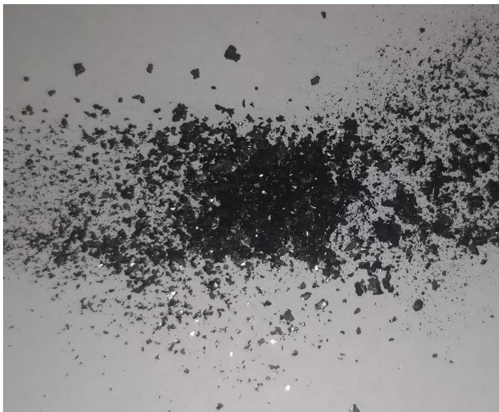
Figure 3.3. SWCNT bucky paper (M-SWCNT) dried in ambient air after purification. The paper has been observed to have torn into pieces during transfer and have high reflectivity.
