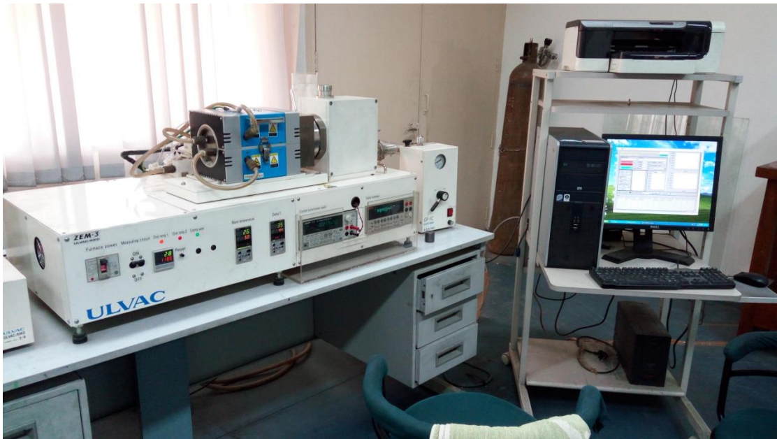
Figure 3.26. ZEM-3 ULVAC RIKO thermoelectric measurement instrument.
