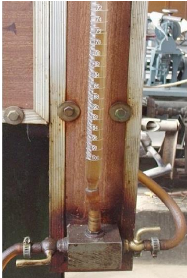
Fig. 3.3 Fuel measuring system (Burette Method)
