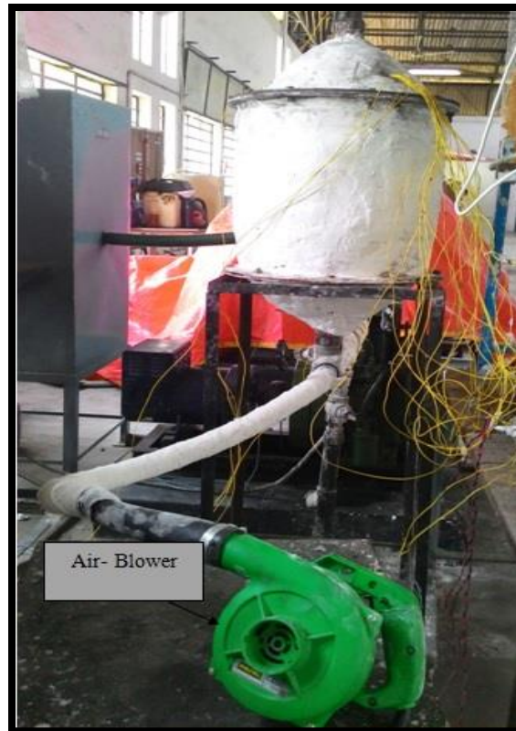
Fig. 3.16 Discharging of TESS
