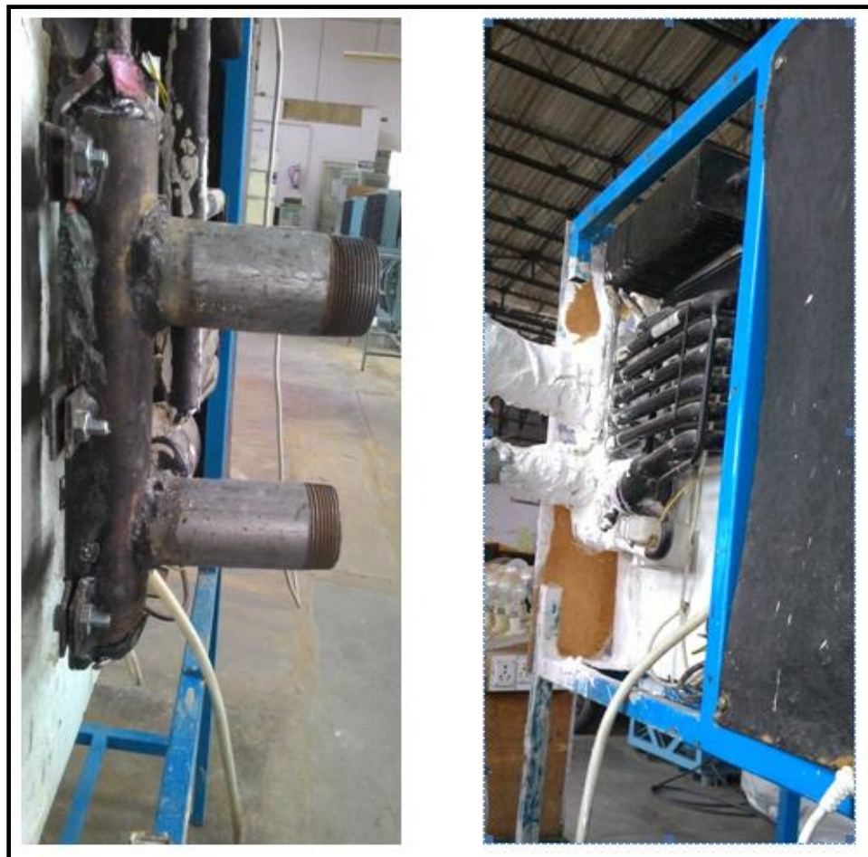
Fig. 3.10 Photographic view of heat exchanger fitted in VA system
