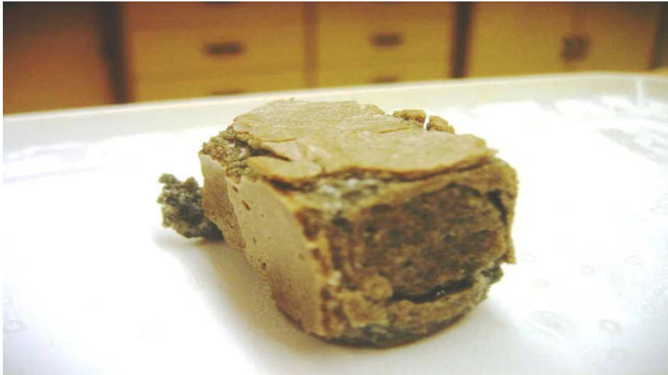
Figure 2.7 Deterioration in Mortar Surface during Sulphate Attack (Ramezaniapour and Hooton, 2013).
