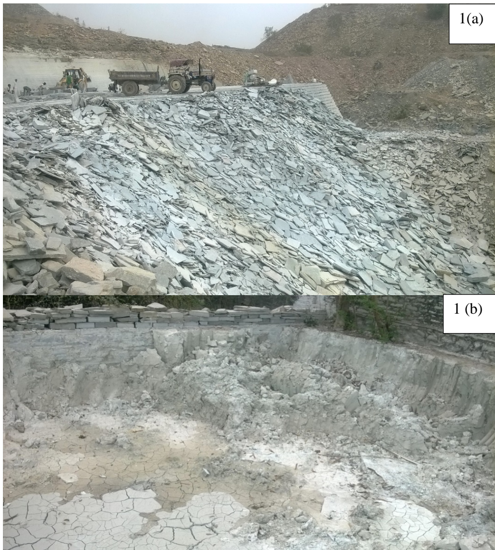
Figure 1.1 (a) and (b): Generated Solid and Slurry Waste from Mining and Processing of Dimensional Limestone.
