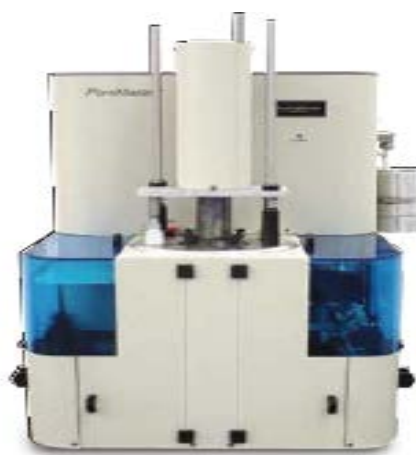
Figure 3.18 Mercury Intrusion Porosimetry Machine (Pore Master - 60 GT)
