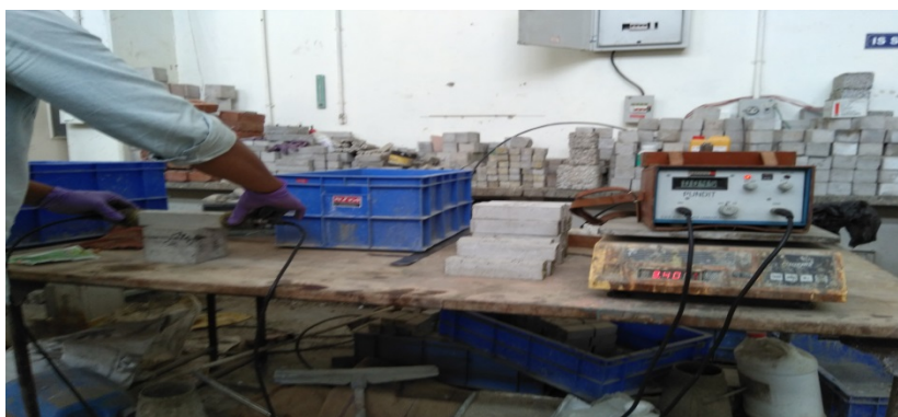
Figure 3.11 UPV Test on Mortar Samples
