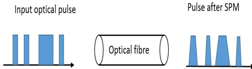
Fig. 2.9 Self phase modulation; reproduced from ref. [100].
