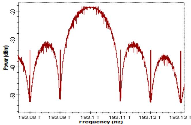
Fig. 3.15 Power spectrum of DPSK
