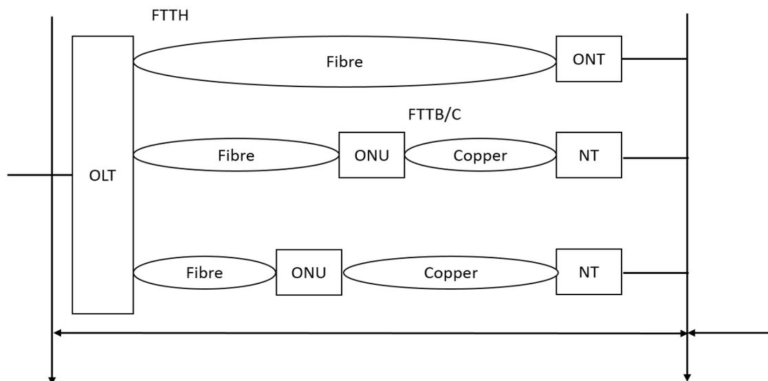
Fig. 1.3 Network Architecture; reproduced from ref. [17].
