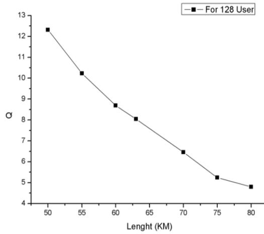
Fig. 4.12 Fiber length vs Q factor for 128 users.
