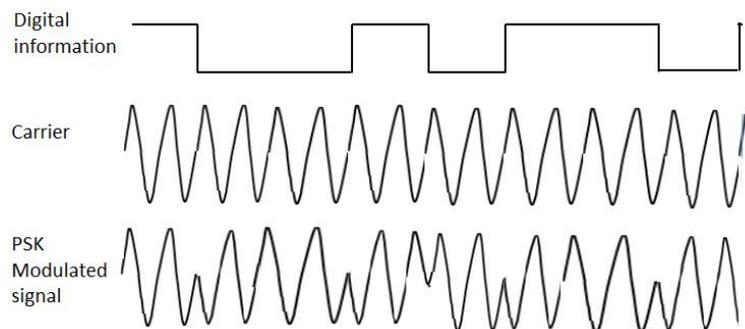
Fig. 3.6 PSK modulation; reproduced from ref. [107].
