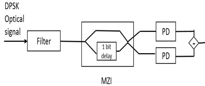
Fig. 3.14 DPSK Receiver circuit; reproduced from ref. [109]
