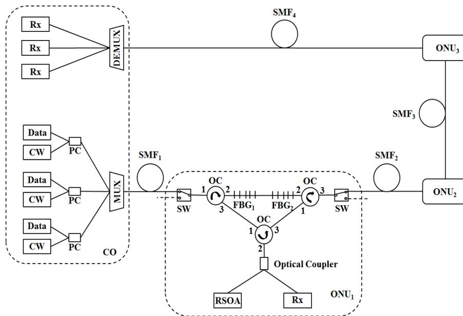
Fig. 5.9 Simulation Setup of dual ring WDM-PON.
