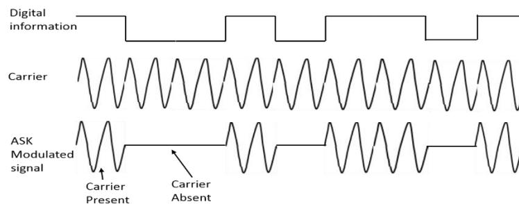
Fig. 3.4 ASK modulation; reproduced from ref. [107].
