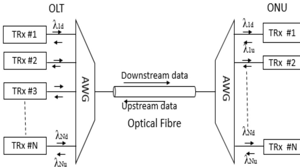
Fig. 2.6 WDM-PON Architecture; reproduced from ref. [82].
