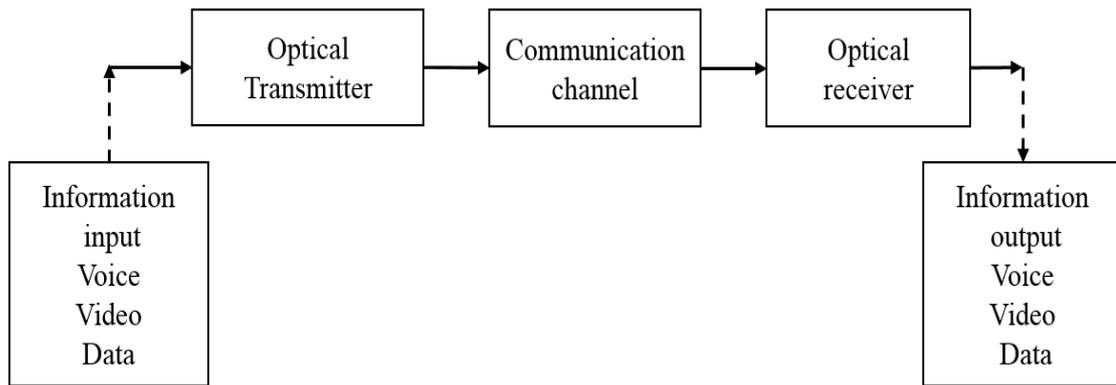
Fig. 1.1 Generalized fiber- optic communication system [5].
