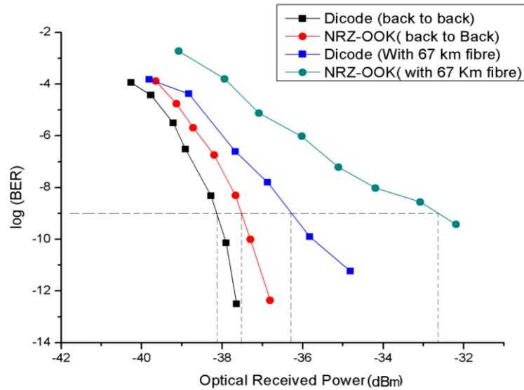
Fig. 6.3 Optical received power vs BER
