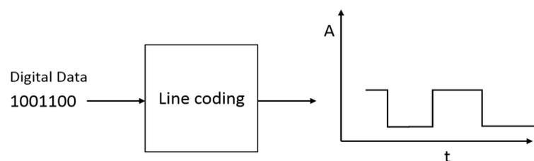
Fig. 3.1 Line coding to convert data to digital signal; reproduced from ref. [42].
