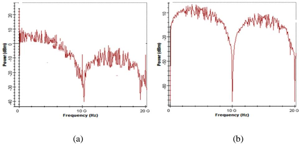
Fig. 3.20 Power Spectra of (a) conventional NRZ (b) dicode-coded NRZ.
