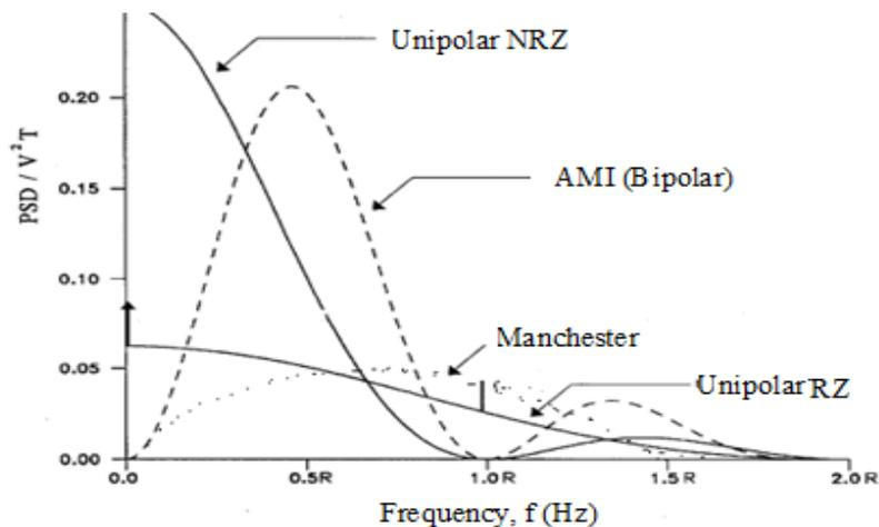
Fig. 3.3 Power spectral density of different line codes; reproduced from ref. [42].
