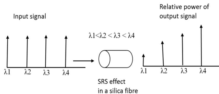
Fig. 2.8 SRS transfer of lower wavelength power to higher wavelength; reproduced from ref. [4].
