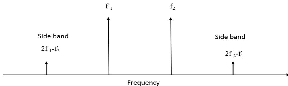
Fig. 2.11 FWM with two signal frequency; reproduced from ref. [4].
