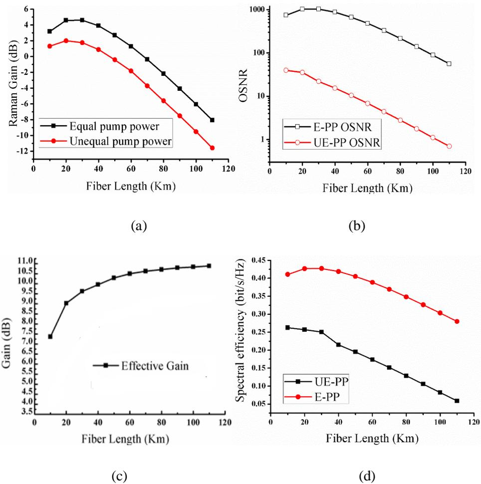
Fig. 4.4 (a) Raman gain, (b) Optical Signal to noise Ratio, (c) Effective Raman gain and (d) spectral efficiency analysis with increasing fiber length.
