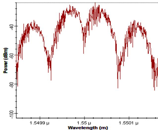
Fig. 4.5 Power spectra of dicode signal.
