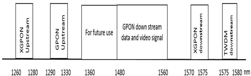
Fig. 2.4 XGPON frequency spectrum band as ITU-T G.987 recommendations; reproduced from ref. [78].
