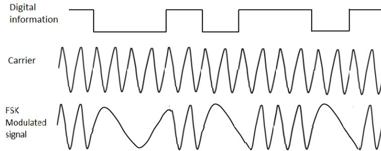
Fig. 3.5 FSK modulation; reproduced from ref. [107].
