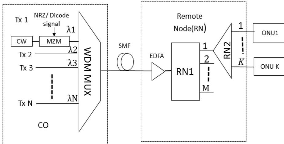
Fig. 6.1 Flexible hybrid PON.
