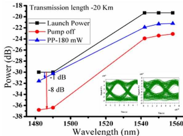
Fig. 4.3 Received power and eye diagram analysis with and without Raman pump.
