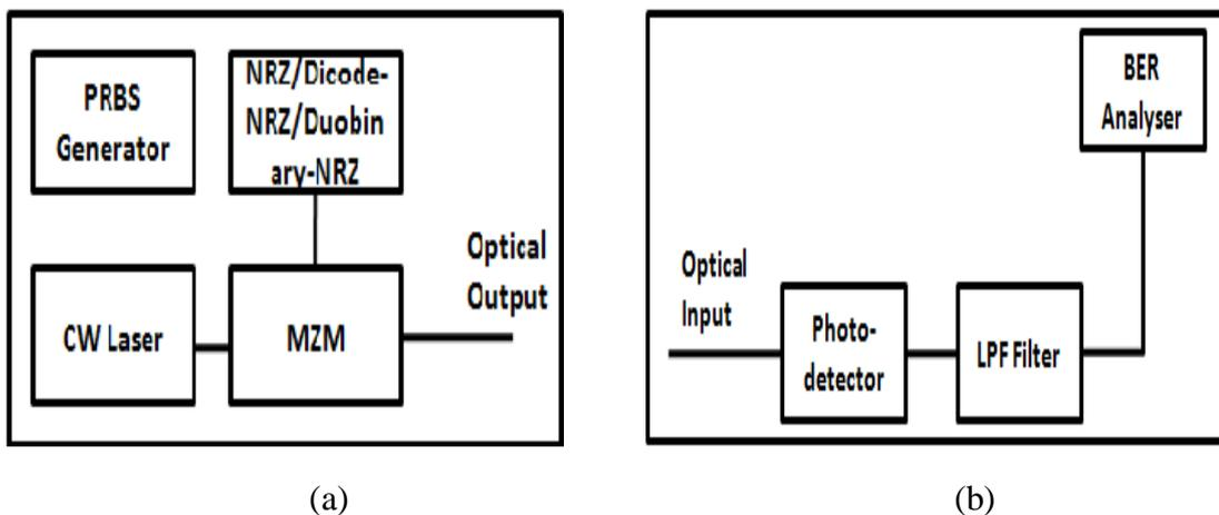
Fig. 5.2 Block diagram of (a) OLT (b) ONU.
