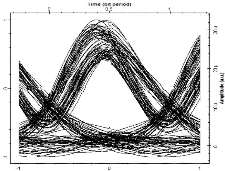
Fig. 5.13 Eye diagram at 40 km for Dicode-coded NRZ.
