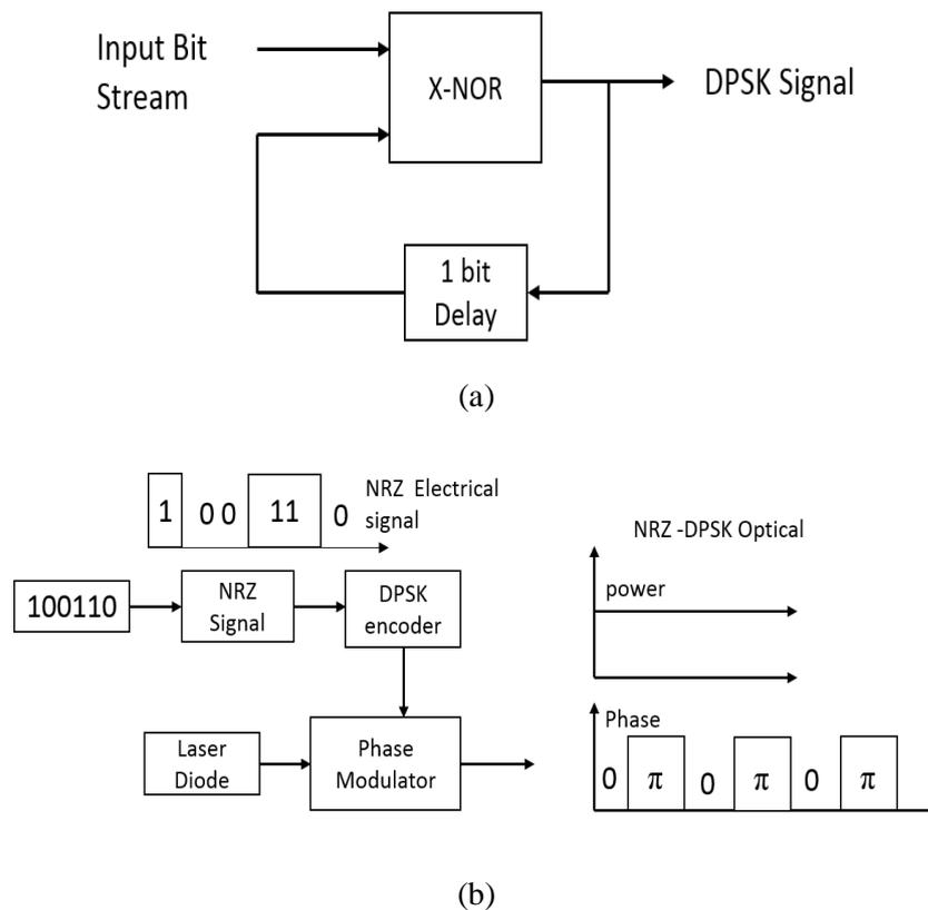
Fig. 3.13 NRZ- DPSK (a) Encoder (b) Modulator; reproduced from ref. [109].
