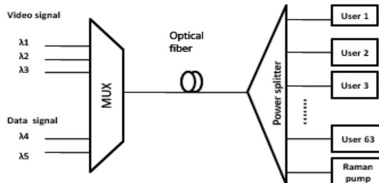
Fig. 4.1 A WDM-TDM system with remote Raman pump
