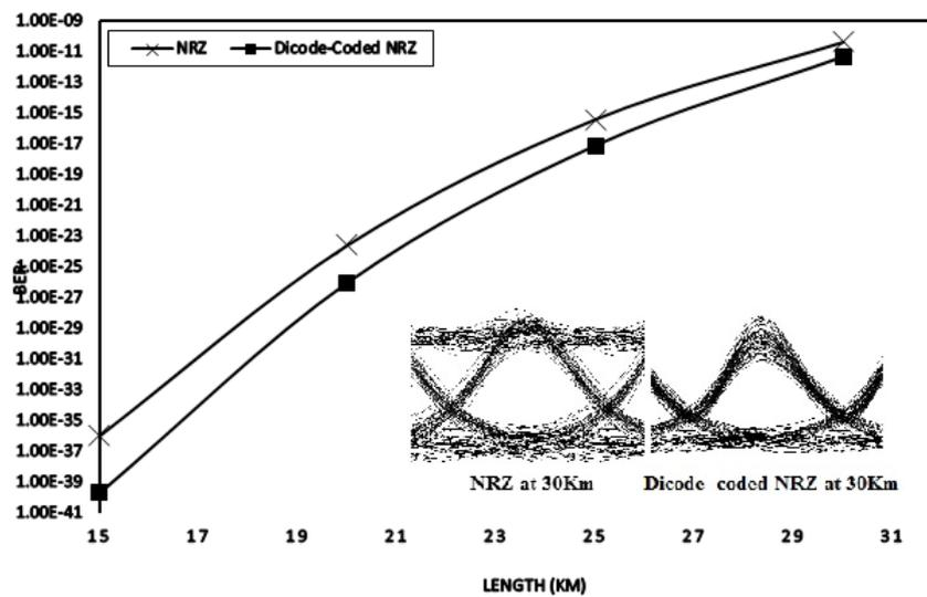
Fig. 5.10 BER performance of NRZ and Dicode-coded NRZ.
