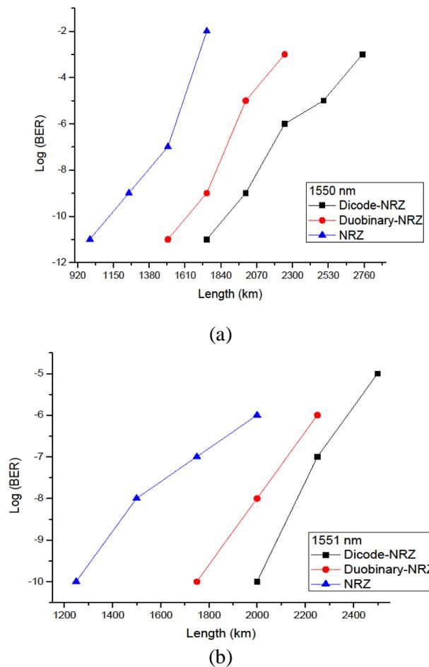
Fig. 5.3 BER performance (a) 1550 nm & (b) 1551 nm
