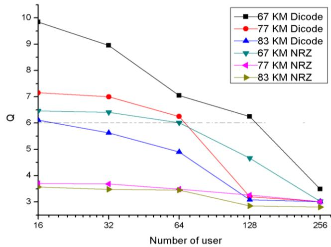
Fig. 6.5 Q factor analysis with length and number of users.
