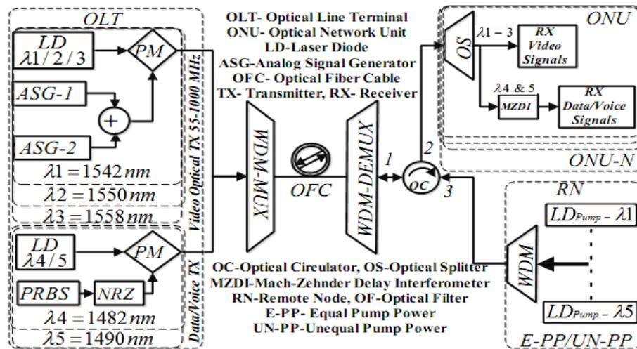
Fig. 4.2 Simulation model of proposed distributed Raman amplified WDM-PON architecture.
