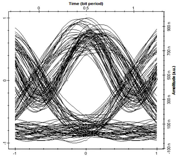
Fig. 4.11 Eye diagram for maximum length for 64 users for 82 KM.
