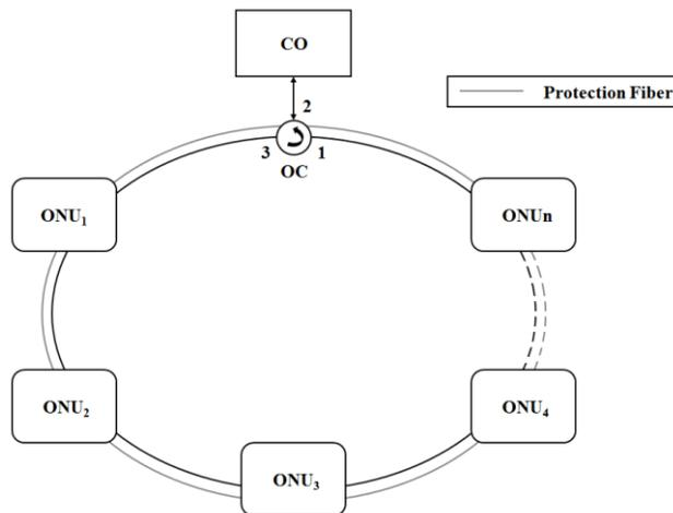
Fig. 5.7 Ring architecture WDM-PON with fibre-fault protection [173].
