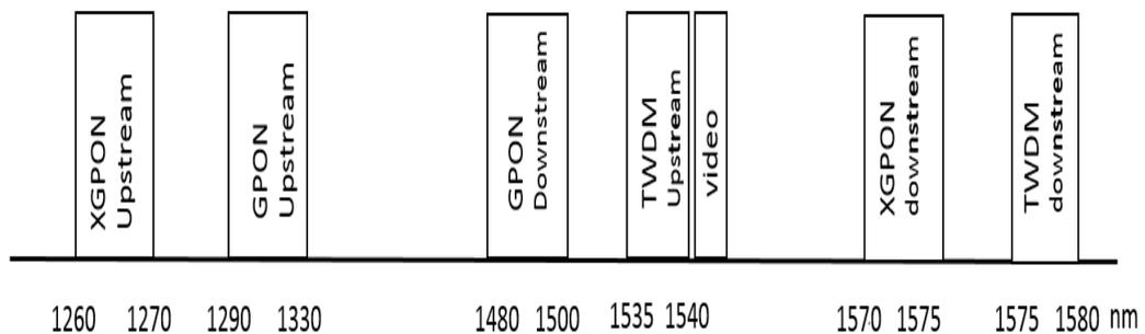
Fig. 2.5 NGPON 2 spectrum band; reproduced from ref. [78].
