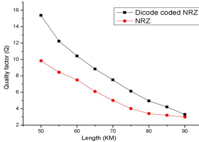
Fig. 6.4 Length v/s Q at 10 Gbps data rate.
