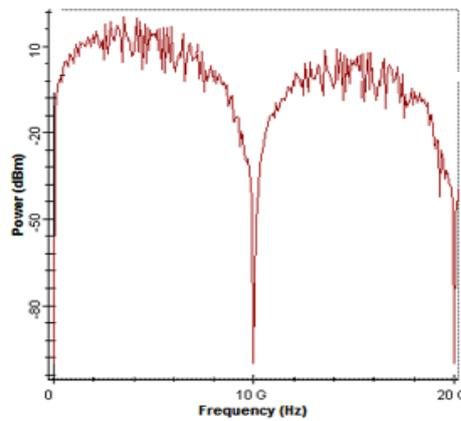
Fig. 5.8 Power Spectra of dicode coded NRZ.
