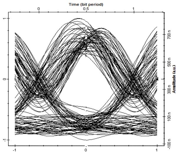
Fig. 4.13 Eye diagram for maximum length for 128 users for 72 KM
