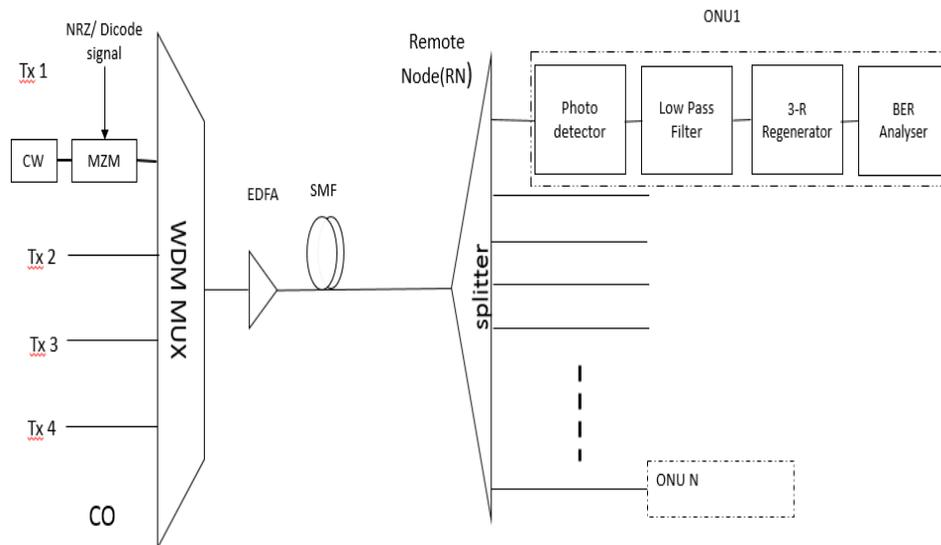
Fig. 4.6 Simulation setup of WDM-TDM-PON.
