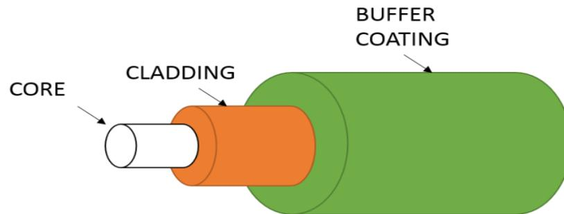
Fig. 1.2 Optical Fiber; reproduced from ref. [4].
