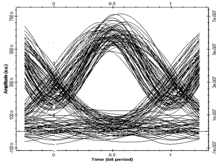
Fig. 6.8 Eye diagram for 128 user at 67 KM for dicode.
