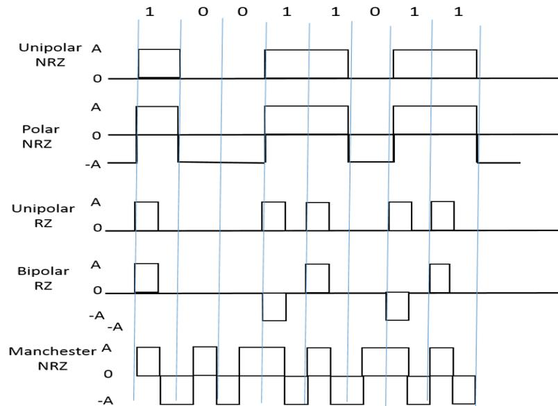
Fig. 3.2 Common line coding; reproduced from ref. [42].
