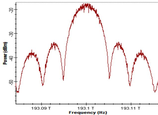
Fig. 3.18 Power spectra of Duobinary after modulation.
