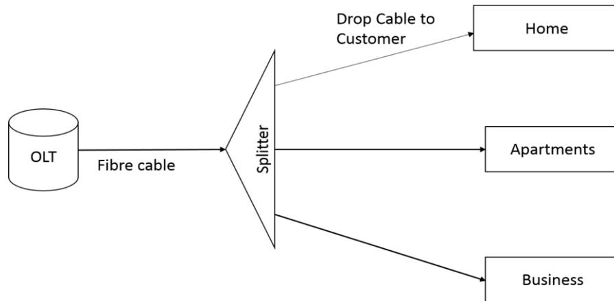
Fig. 2.1 Basic PON architecture,
