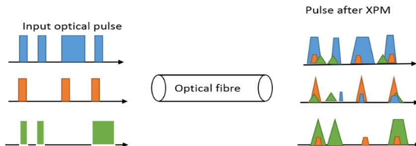
Fig. 2.10 Cross phase modulation; reproduced from ref. [102].
