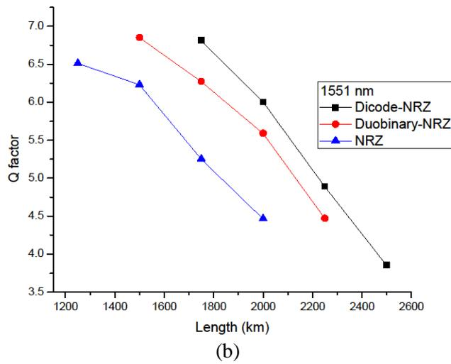
Fig. 5.4 Q factor performance (a) 1550 nm & (b) 1551 nm
