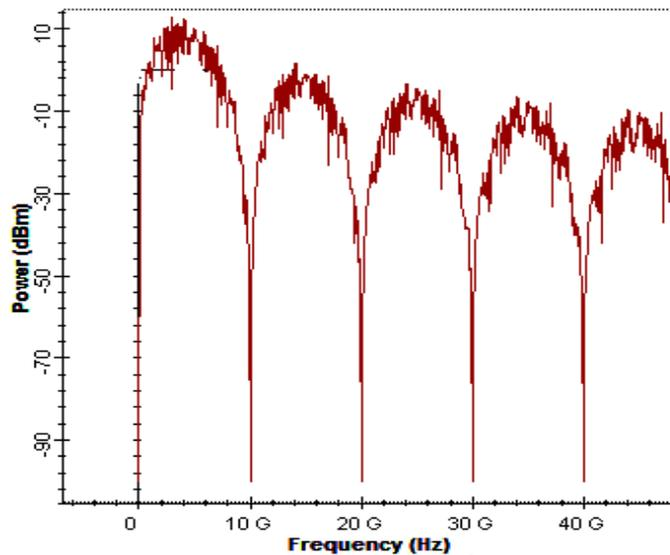
Fig. 4.7 Electrical Dicode signal.
