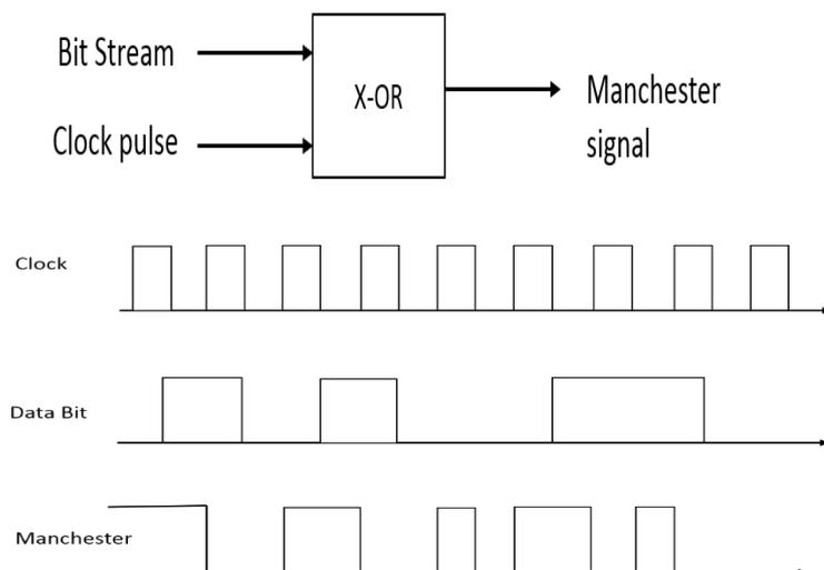
Fig. 3.11 Binary to Manchester generation of waveform; reproduced from ref. [42]
