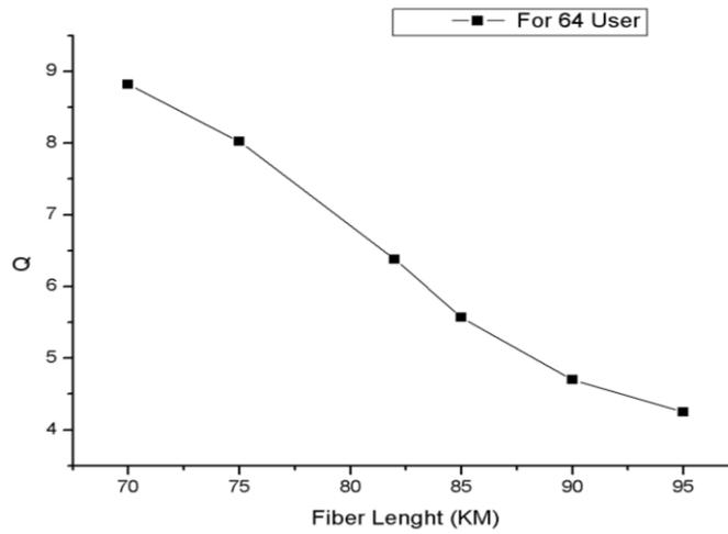
Fig. 4.10 Fiber length vs Q factor.
