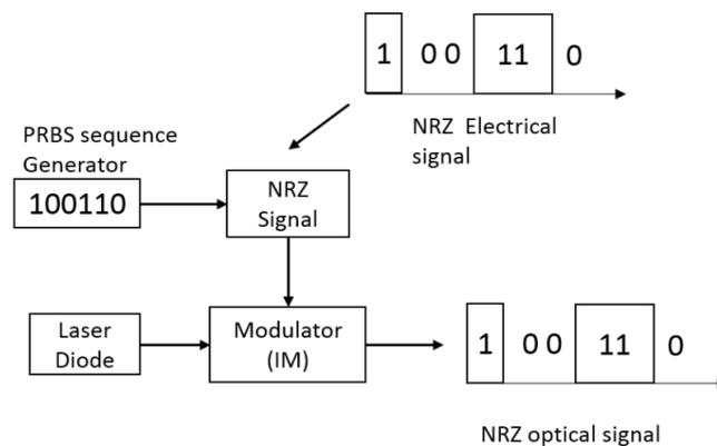
Fig. 3.7 NRZ- OOK transmitter; reproduced from ref. [109].
