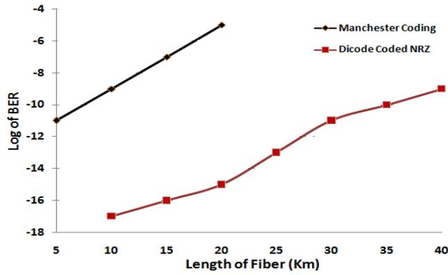
Fig. 5.12 BER Performance of Manchester and Dicode coded NRZ.
