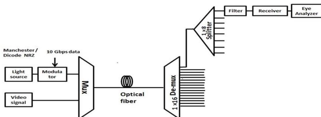
Fig. 5.11 Simulation Setup of HPON.
