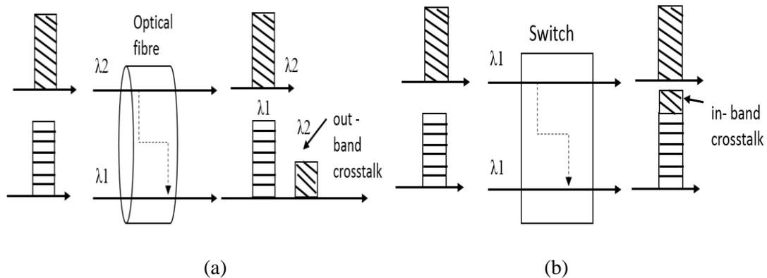
Fig. 2.7 (a) Out-band cross talk (b) in-band cross talk; reproduced from ref. [95].
