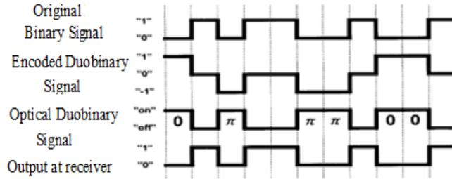
Fig. 3.17 Generation of Duobinary waveform [118].
