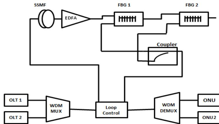
Fig. 5.1 Simulation setup of FBG post compensation.
