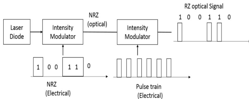
Fig. 3.9 Block diagram of a RZ transmitter.
