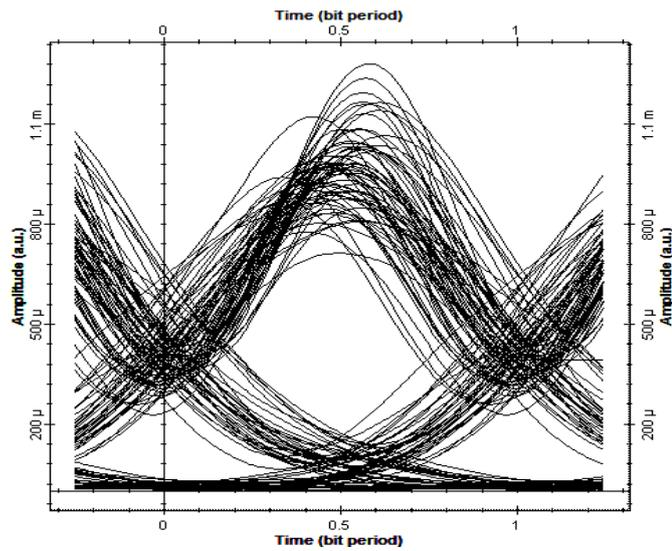
Fig. 5.5 Eye pattern of Dicode-NRZ scheme with FBG for 2000 Km
